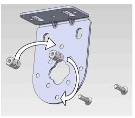
Bracket with the two pins installed as shown on the picture on the right side is used for wall mount installations. Please make sure that motor rests on both pins during installation.
