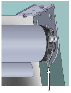
Secure motor in the bracket with the wire clip
