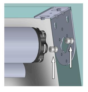
Motor slides into 2 pins on the brackets Pins should always be in horizontal position.
