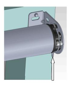
Secure motor in the bracket with the wire clip
