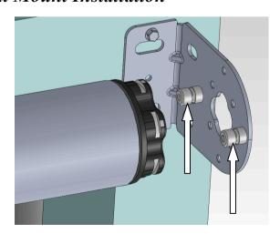
Motor slides into 2 pins on the brackets Pins should always be in horizontal position.
